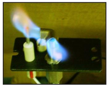
Figure 3.1 IPI Pilot Flame Patterns
